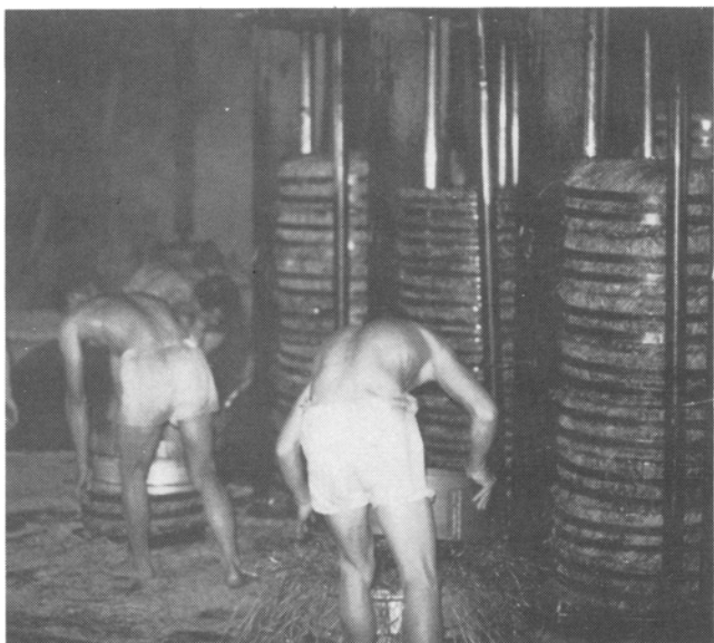
FIG. 1. This old-fashioned oil expressing plant is one of 124 oil refineries in Taiwan.
